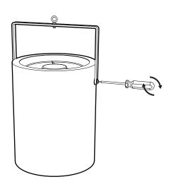
The Designer Series system is designed to hang vertically and freely 12-to-18 inches, or as close as possible, from the ceiling on professionally installed hardware, for models 10/15/25, capable of supporting a minimum of five times the weight of the Designer Series unit, 60 lb. (27 kg.). Example - 1/4" (7 mm) diameter steel bolt is rated at 60 lb. (27 kg.) load.
