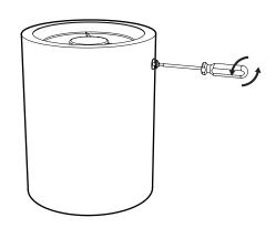
2 Swing the bail to the vertical position and tighten the two Torx screws.
