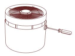
2 Swing the bail to the vertical position and tighten the two Torx screws.
