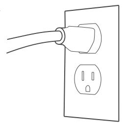
**G**NOTE: SECURE the power cord to the ceiling structure as added security. The cord will act as a safety leash and by securing it the possibility of the plug accidentally coming out of the outlet in the future is greatly reduced. A 50 lb. (20 kg.) rated Zip-Tie or mechanics wire are examples of methods of securing the power cord.
