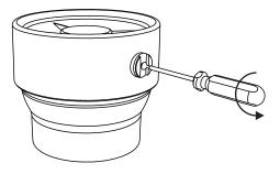
2 Swing the bail to the vertical position and retighten the two Torx screws.
