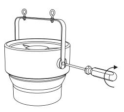
**3** The Pearl system is designed to hang vertically and freely 12-to-18 inches, or as close as possible, from the ceiling on professionally installed hardware capable of supporting a minimum of five times the weight of the Pearl unit. Example - 1/4" (7 mm) diameter steel bolt is rated at 60 lb. (27 kg.) load.
