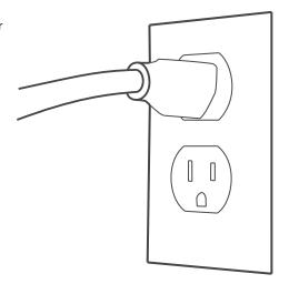
NOTE: SECURE the power cord to the ceiling structure as added security. The cord will act as a safety leash and by securing it the possibility of the plug accidentally coming out of the outlet in the future is greatly reduced. A 50 lb. (20 kg.) rated Zip-Tie or mechanics wire are examples of methods of securing the power cord.
