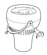
$2^{\hbox{Swing the bail to the vertical position and retighten the two Torx screws.}$
