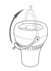
The PureAir system is designed to hang vertically and freely 12-to-18 inches, or as close as possible, from the ceiling on professionally installed hardware, for models 10/15/25, capable of supporting a minimum of five times the weight of the Air Pear unit, 60 lb. (27 kg.). Example - 1/4" (7 mm) diameter steel bolt is rated at 60 lb. (27 kg.) load.
