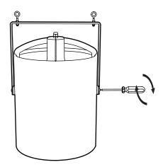
The Q Series system is designed to hang vertically and freely 12-to-18 inches, or as close as possible, from the ceiling on professionally installed hardware capable of supporting a minimum of five times the weight of the Q Series unit, 60 lb. (27 kg.). Example - 1/4" (7 mm) diameter steel bolt is rated at 60 lb. (27 kg.) load.
