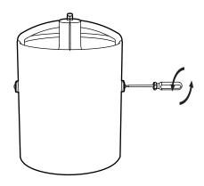
2 Swing the bail to the vertical position and tighten the two Torx screws.
