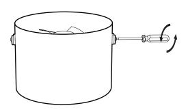
2 Swing the bail to the vertical position and tighten the two Torx screws.
