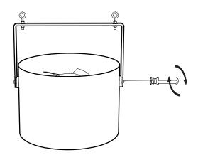
The Retail Series system is designed to hang vertically and freely 12-to-18 inches, or as close as possible, from the ceiling on professionally installed hardware, for models 10/15/25, capable of supporting a minimum of five times the weight of the Retail Series unit, 60 lb. (27 kg.). Example - 1/4" (7 mm) diameter steel bolt is rated at 60 lb. (27 kg.) load.
