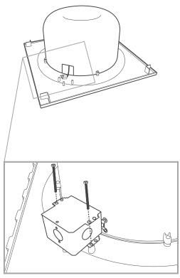
The base has four right angle tabs located at each corner that can be drilled for additional ceiling/support wires to be added if desired.
